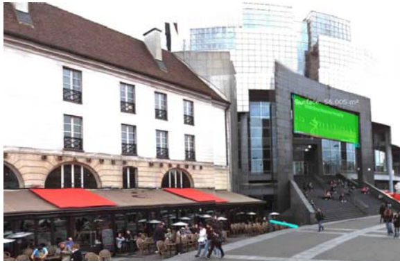
Figure 5: One click surface measurement over a large advertising panel shows the square meters of the surface selected.
