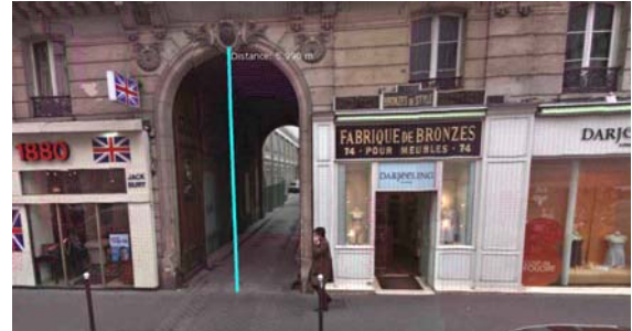
Figure 1: A screenshot of the web application while measuring the height of a porch with the laser cloud visualization activated.
